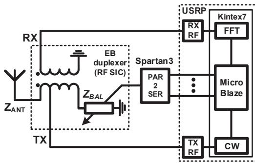
Fig. 2. Platform block diagram
