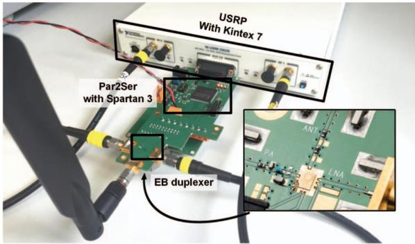
Fig. 1. Hardware overview showing the USRP, interfacing PCB and EBD
