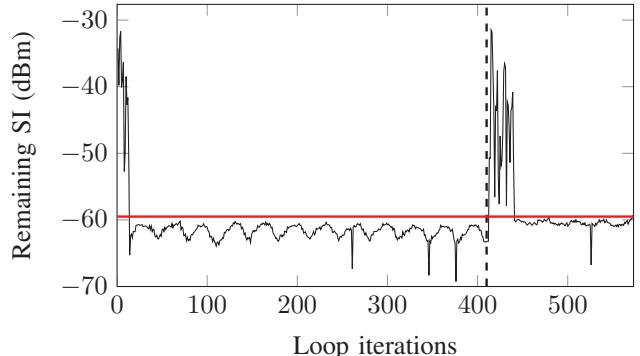
Fig. 3. Remaining SI after EBD cancellation. (—) is the threshold of the PSO algorithm and (---) indicates when the antenna impedance changes.
