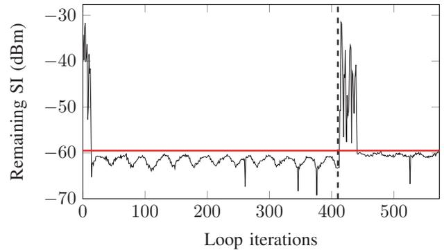
Fig. 3. Remaining SI after EBD cancellation. (—) is the threshold of the PSO algorithm and (- -) indicates when the antenna impedance changes.
