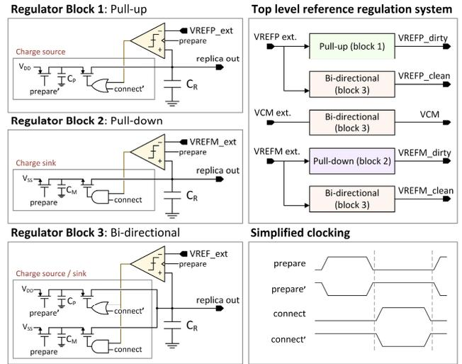
Fig. 1: Fully dynamic, discrete-time reference regulation system.
