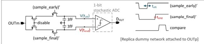
Fig. 3: Ring amplifier and attached “scope-on-chip” monitor.
