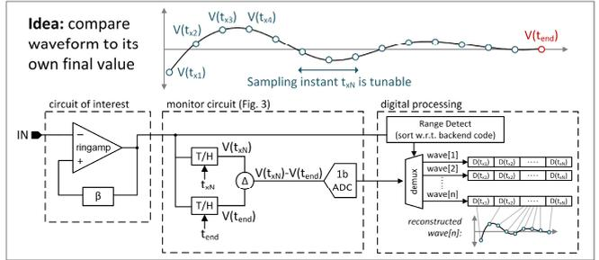
Fig. 4: Concept of amplifier settling waveform reconstruction.
