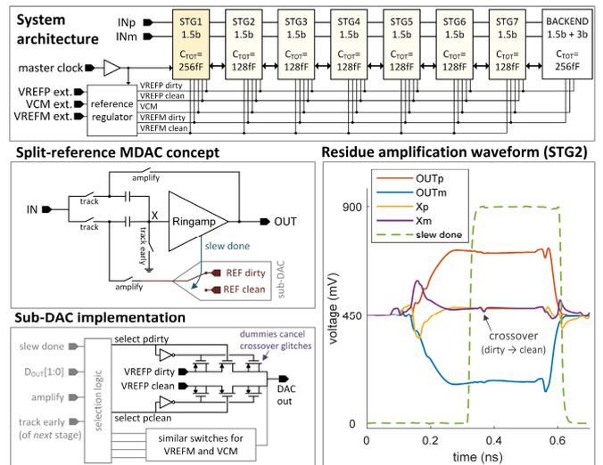
Fig. 2: Integration of regulation system into the ADC.
