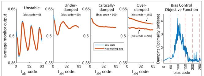
Fig. 5: Measured performance of regulator and ringamp monitor.
