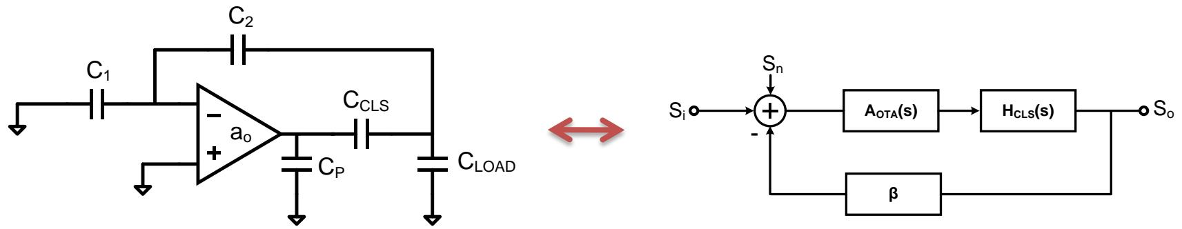
$$H_{\text{CLS}}(s) = \frac{C_{\text{CLS}}}{C_{\text{CLS}} + C_{\text{LD}}} \quad (3)$$
