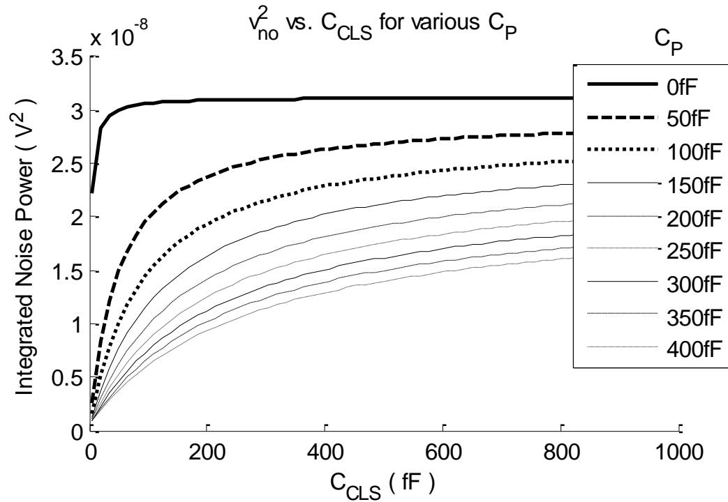
$$C_P \gg \frac{C_{CLS} \cdot C_{LD}}{C_{CLS} + C_{LD}} \rightarrow C_{CLS} \text{ and noise are heavily correlated.}$$
