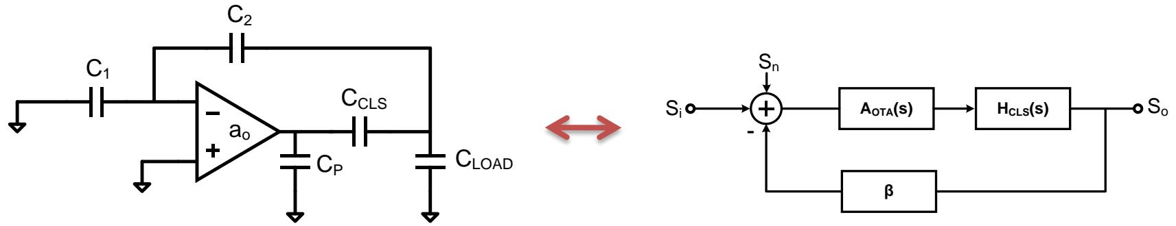
When 1/f noise is entirely in passband of  $A_{OTA}(s)$ , noise sources can be treated as frequency-independent constants:
